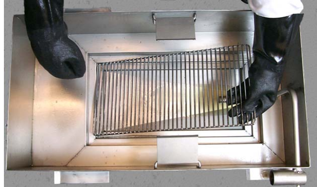
Placing filter screen (pan grid) in filter pan.
